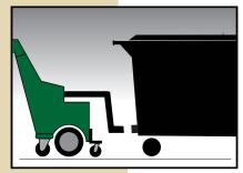
Insert tube on the front of the WasteCaddyLite attaches to the bottom of the dumpster.
